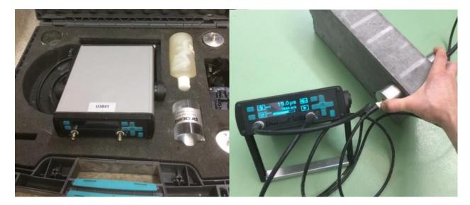
Photo 4 Ultrasonic testing equipment
