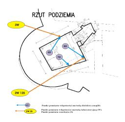
Fig. 14 Sampling points for tests on the ground floor of the defensive tower of the Janowiec castle
