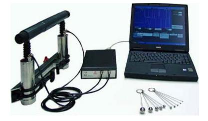
Fig. 7 Hammer test set (source: http://www.impact-echo.com/Impact-Echo/images/wssetup.jpg)
