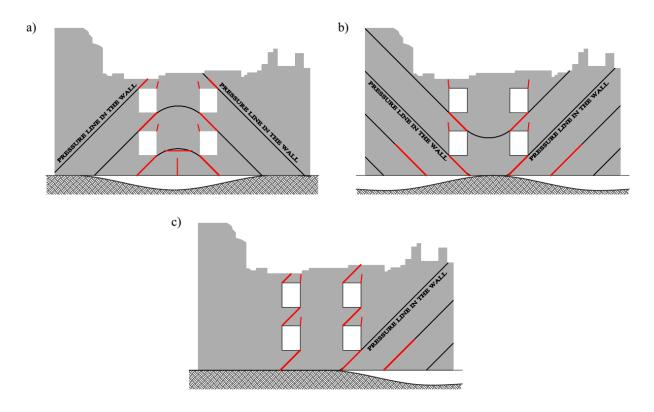
Fig. 3. The ideological course of the pressure line and damage in the wall due to: - a) settlement of the central part of the wall, b) settlement of both wall corners, c) settlement one of the corners [3]
