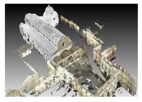
Picture 7: example of laser scan technology applied on a monumental complex
