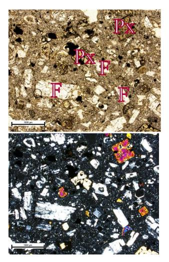
Fig. 6, 7 Detail of feldspars (F) and pyroxen (Px) phenocrysts (parallel polars and the same in crossed polars)
