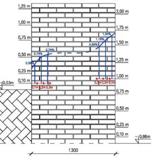
Fig. 16 Diagram of the distribution of salinity with sulphates at the level of the cellar wall at the sampling from the depth of 0.1 m.
