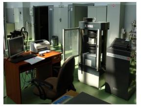
Photo 8 Test stands - the Controls Advantest 9 hydraulic press
