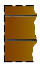
Fig. 9 Salt corrosion of the wall surface with mortar weaker than the masonry material.
