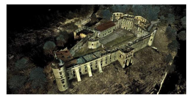
Fig. 1 The cloud of points, which was created as a result of the preparation of spatial data obtained from the Leica C10 scanner.
