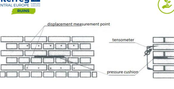
On the basis of measurements, the stresses in the wall by means of the formula are determined:
