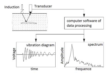
Fig. 6 Scheme of the test 0
