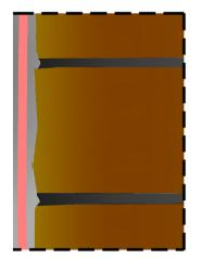
Fig. 12 Salt corrosion inside the plaster layer
