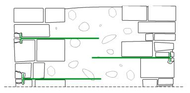
Fig. 9. Scheme of nailing with the supplementation of the wall's face of the "opus emplectum" type
