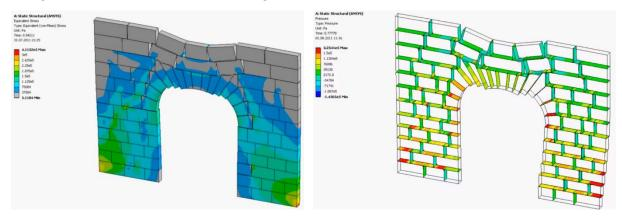
Fig. 18 View of stresses in a wall element and joints (source: https://i.ytimg.com/vi/sMpNE9L2reY/maxresdefault.jpg)
