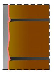
Fig. 11 Salt corrosion at the interface between plaster and masonry
