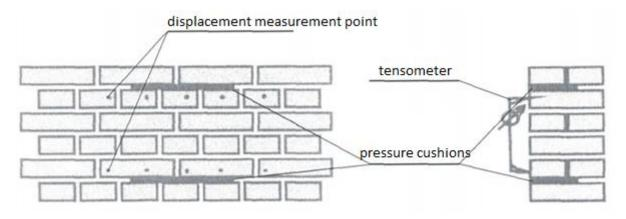
In order to obtain the result of the compressive strength of the wall, it is necessary to put pressure in the cushions to cause local destruction of the masonry structure. The destructive pressure will be the limit strength of the masonry structure. Destruction is not reversible, and the test becomes a destructive test.
