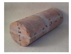
Photo 6 Core through the thickness of the wall. 0
